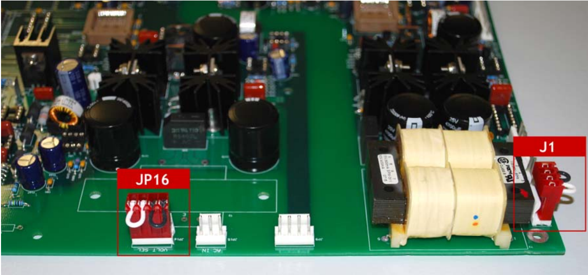
Figure 2. 100-120 Vac Jumper Settings
