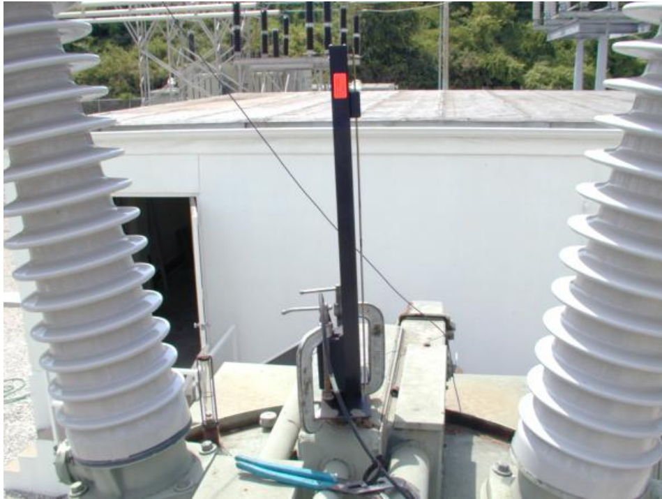
Linear Transducer on an OCB
